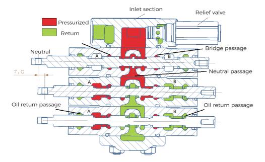
For multi-section valves, if one of the section spool is in left or right position, there is no flow in its down stream section neutral passage. The main throttle occurs on the valve opening between bridge passage and spool. The operator can control more than one spools, but the flow rate for each controlled section depends on the load.
