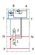
GKV80 series sectional valve is an open circuit 3-position 4-way valve. When spool is in its neutral position, the flow from pump passes through the neutral passage to tank, with very low pressure drop. When one of the spool is moved to 1 or 2 position, the neutral passage is blocked. The flow from pump can only pass though parallel passage to load check valve, go through the bridge and spool opening to work port A or B.
