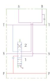
GKVL80 series sectional valve is an open circuit 3-position 4-way valve. When spool is in its neutral position, the flow from pump passes through the neutral passage to tank, with very low pressure drop. When one of the spool is moved to 1 or 2 position, the neutral passage is blocked. The flow from pump can only pass though parallel passage to load check valve, then go through the bridge and spool opening to work port A or B.
