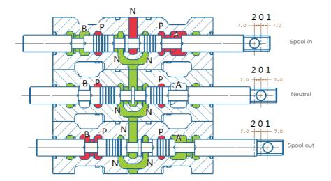
For multi-section valves, if one of the section spool is in 1 or 2 position, there is no flow in its down stream section neutral passage. The main throttle occurs on the valve opening between bridge passage and spool. The operator can control more than one spools, but the flow rate for each controlled section is dependent on the load.
