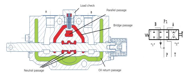
GKV35 series sectional valve is an open circuit 3-position 4-way valve. When spool is in its neutral position, the flow from pump passes through the neutral passage to tank, with small pressure drops. When one of the spool is moved to LEFT or RIGHT position, the neutral passage is blocked. The flow from pump can only pass the parallel passage to load check valve, then passes through the bridge and spool opening to work port B or A.
