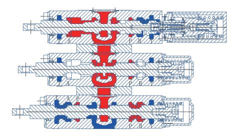
For multi-section valves, if one of the section spool is in 1 or 2 position, then there is no flow in its down stream section neutral passage. The main throttle occurs on the valve opening between bridge passage and spool. The operator can control more than one spools, but the flow rate for each controlled section is dependent on the load.
