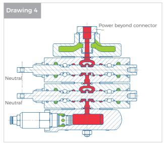
For multi-section valves, if one of the sections spool is in 1 or 2 position, there is no flow in its down stream sections neutral passage. The main throttle occurs on the valve opening between bridge passage and spool. The operator can control more than one spool, but the flow rate for each controlled section depends on the magnitude of the load, as shown in drawing 3.
