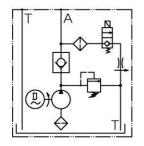
This hydraulic power unit is made up of high pressure gear pump, AC motor, multi-manifold, hydraulic valve, oil tank, etc. It used at the power origin of light fork truck and pallet truck. Electromagnetic unloading valve unloading to oil return, decline speed is controlled by pressure compensating flow control valve.
