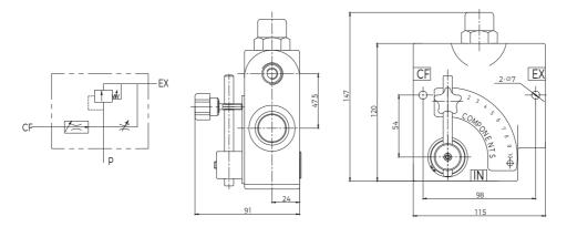
LKF model is a full range pressure compensating variable flow control. It is designed so that the orifice area varies as the lever is rotated. The outlet flow is smooth and constant regardless of the pressure on the control flow or excess flow ports. An adjustable ball spring relief allows for pressure compensated flow up to the pressure setting on the relief. Relief valves are preset at 1500 psi and adjustable range from 750 to 3000 psi.
